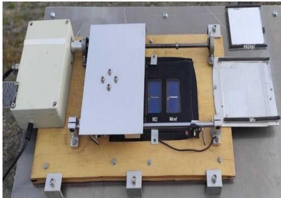
Fig.1: Left: Soiling sensor by CIEMAT-PSA. Right: Soiling sensor by Tekniker.
