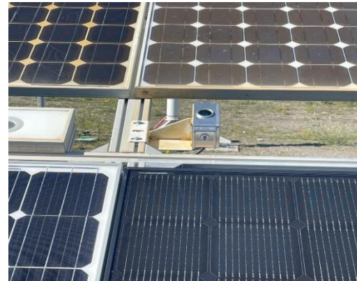
Fig.1: Left: Soiling sensor by CIEMAT-PSA. Right: Soiling sensor by Tekniker.
