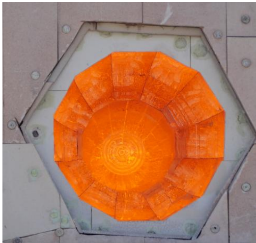
Fig. 1: Receiver operating at 1200°C in the SSPS tower of the Plataforma Solar de Almería in Tabernas (Spain).
