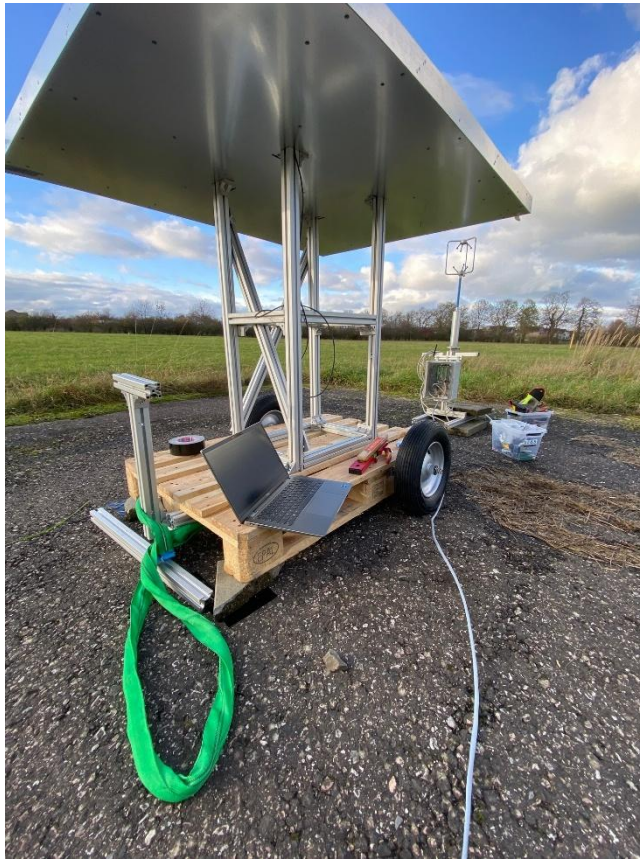
Fig.1: Left: simultaneous measurements using the ultrasonic anemometer and the rigid measurement plate; Top right: Normalized frequency spectrum of the vertical wind component; Bottom right: distribution of differential pressure time series across the plate.
