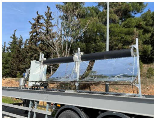
Fig. 2: Preliminary design of a pilot-scale mobile HTL reactor with parabolic troughs
